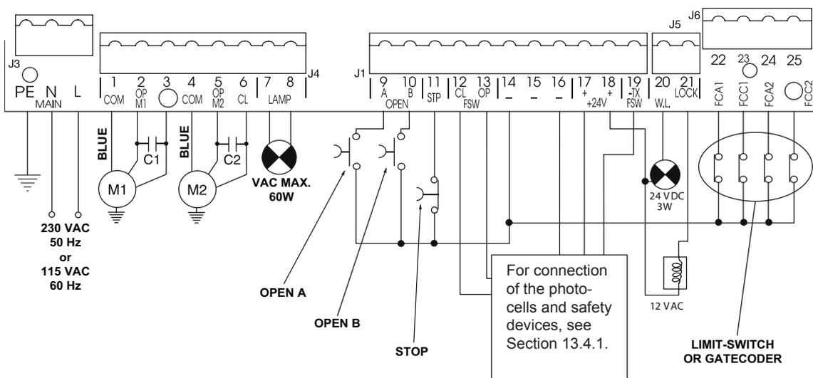
NB: Capacitors are supplied with the operator.
