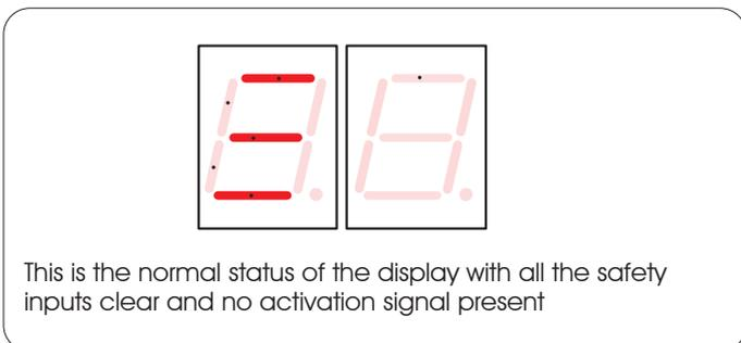
This is the normal status of the display with all the safety inputs clear and no activation signal present
