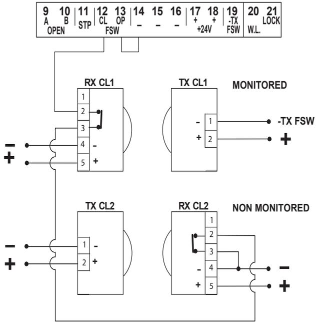
**Connection of a pair of Monitored Closing Photocells, and one pair of Non Monitored Opening/Closing Photocell**
