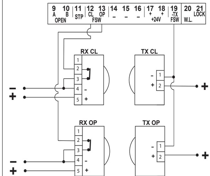
If an additional monitored opening safety device is needed it can be connected to the STP input. The "OP" parameter in the board configuration must be set to active
