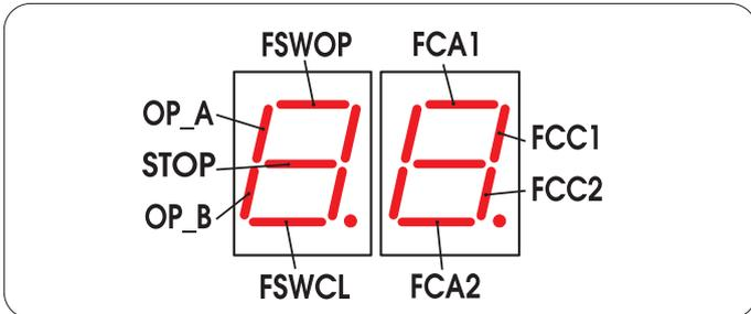
The table below shows the status of the LEDs in relation to the status of the inputs.
