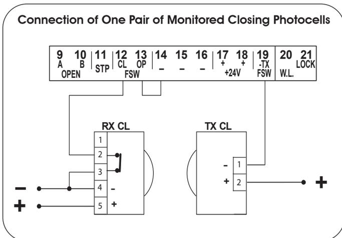
Monitoring of the opening safety devices must be enabled in the board configuration. To enable it enter in advanced programming by pressing and holding "F" and then press "+", scroll to the "FS" parameter and select "Active".
