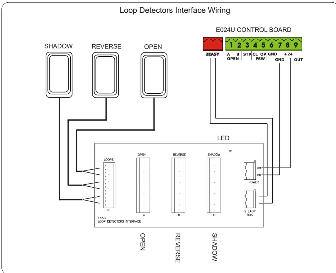
**NOTE:** You can use the shadow loop interface OR the loop detectors interface but not both at the same time. If two monitored open safeties are required the additional loop detectors (other than the shadow) must be wired directly to the E024U board.
