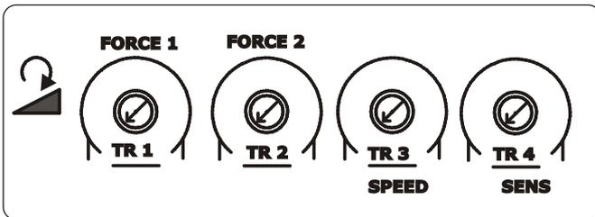
1. Apply resistance to the gate and adjust the Force to make sure that the operator creates enough thrust to reliably move the leaf.
