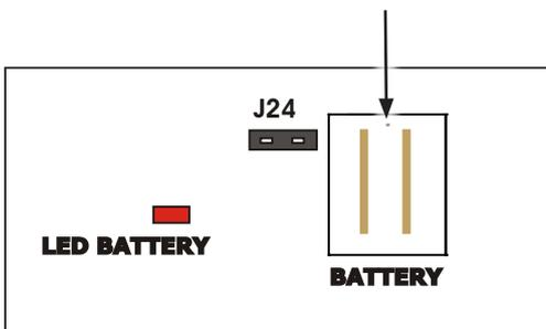
Then turn ON the Battery switch on the top right of the enclosure
