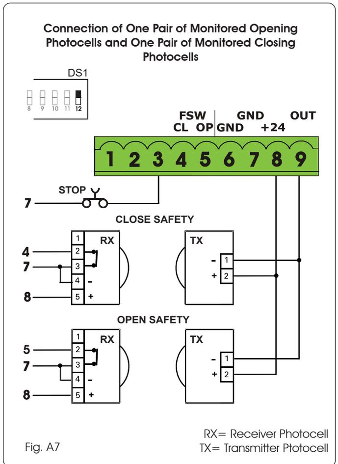
Only one monitored photocell can be connected to the Closing or Opening safety inputs. More than one photocell or other device can be connected to the safety inputs, but they will not be monitored.
