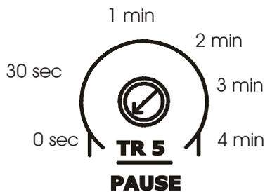
Dip switches DS1: 1 to 3 need to be set for an operating mode with PAUSE time for this adjustment to have any effect
