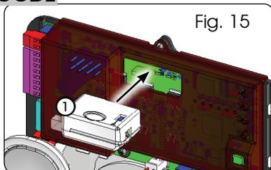
**☞ The 3 types of radio coding (DS, SLH, LC/RC) can co-exist at the same time on the two channels. It is possible to enter up to 256 radio codes subdivided between OPEN A and OPEN B.**
