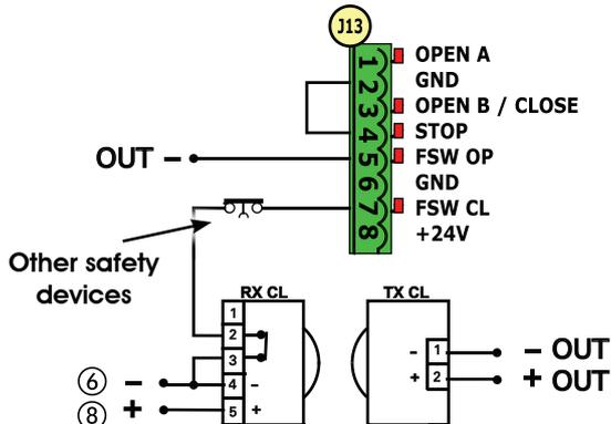
Connection of 1 pair of closing photocells with FAIL-SAFE and STOP safety device **deactivated**
