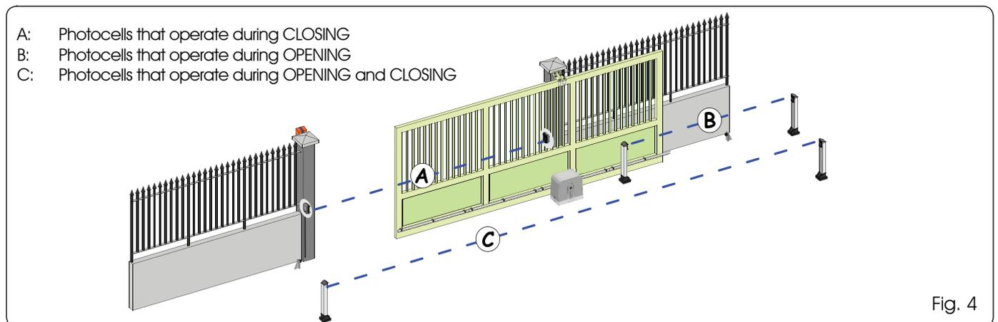
Before connecting the photocells, it is advisable to select the type of operation on the basis of the area of movement that they need to protect:
